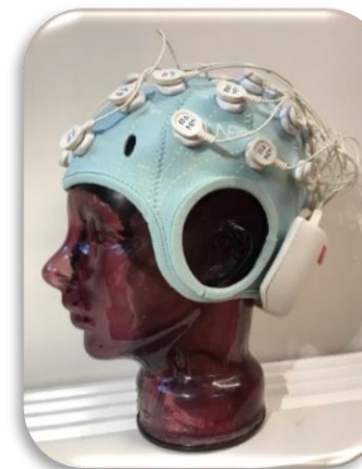
Fig. 2 HD-tDCS equipment, Starstim 32 (Neuroelectronics, Spain)
