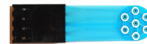
Figure 6: A new planar concentric array electrode design with 7 interconnected anode-cathode pairs. The electrode has a size of 3.8 cm x 0.99 cm. The anode width is 0.3 mm, the cathode radius 0.25 mm, and the anode-cathode distance is 0.5 mm.
